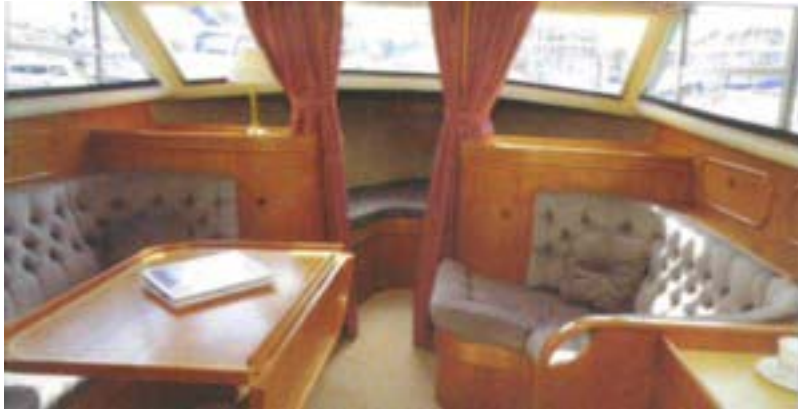
Power Game II's accommodation is plush, with comfortable upholstery, plenty of teak-faced Bruynzeel plywood and solid teak fiddles.
